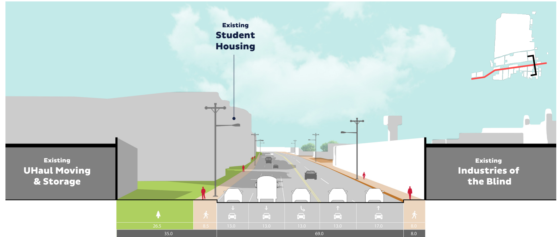
Gate City Boulevard Street Section - Existing
